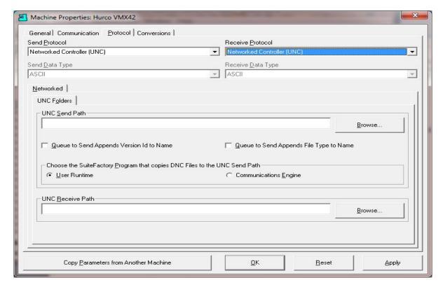
For both the UNC Send Path and UNC Receive Path click Browse and enter the path to the share folder on the CNC. Using the CNC's IP address is the most direct way to its shared folder. You can use the CNC's computer name if it is on a network with DNS (Domain Name System) services. Click Browse and enter the path manually. Note! The OK button will not be enabled unless the path you've entered actually exists.
