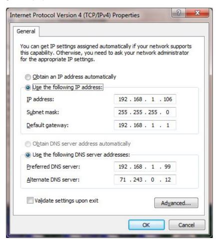
The above is an example. You must set this up as per the requirements of your own network. It could be setup to obtain an IP address automatically or to use a specifically assigned unique address. We recommend an assigned address. Then you can use that IP address to access the CNC rather than trying to find it by a name.
