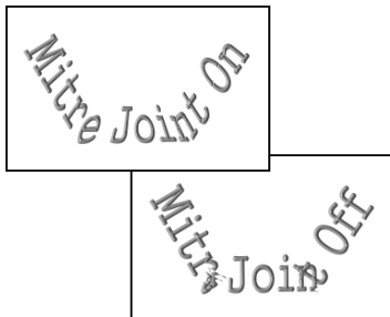
Above: Mitre Joint Below: Without Mitre Joint
