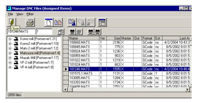
Click Close and you return to the Monitor Screen. But now the DNC File you selected in shown. You now go to your Machine Controller and select the Read function. Last Data Transferred will show the program data being sent and a progress bar keeps track of how much data was transmitted. If most of the time you know the name of the file you need, then leave this window on your computer screen ready to select the next machine and/or DNC file you need.
