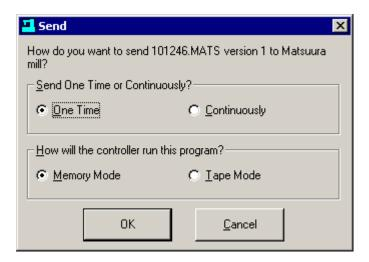
Click OK unless you are drip-feeding to the CNC in real time (Tape Mode). In Memory Mode a timeout is active which clears the file from the machine queue if the data transfer is stopped by the CNC for the set amount of time. (A SuiteFactory parameter). In Tape Mode this timeout is ignored so that the file stays on the queue during long cutting of arcs for example. Selecting "Continuously" causes the file to be re-queued each time it's sent for doing production jobs in Tape Mode.
