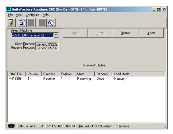
At the CNC, V48VTL output (punch, send . . .) the file. As the data is received the Received 0 bytes field will be updated. When done the file will be removed from the queue automatically after about 5 seconds.
