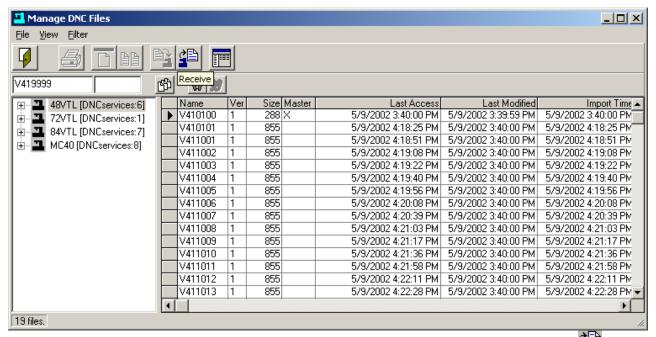
The machine 48VTL is selected. Enter a new file name, V41999, in this example, and the Receive button is enabled.
